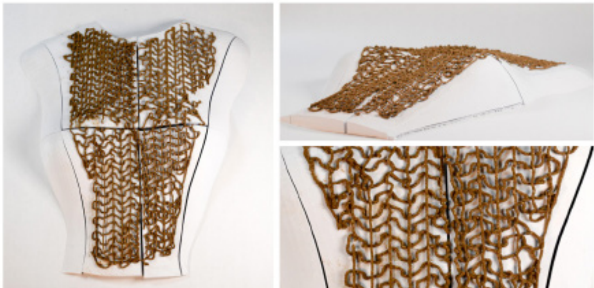
Figure 9: Auxetic geometry 2 printed on torso terrain with agar earth-fiber mix.
